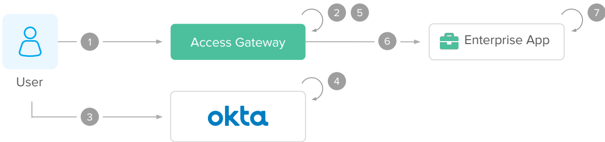
Conceptual Architecture: Header-based Authentication with Okta (SP initiated flow)
